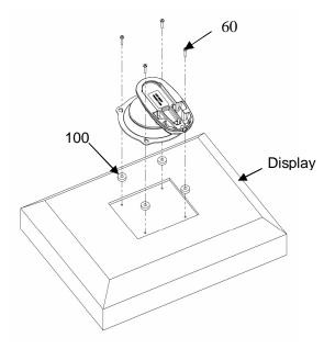
Figure 3. Recess Mount Centris Bracket to Display
